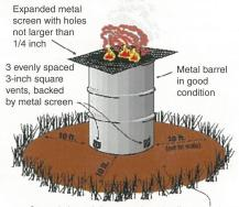
Ground cleared down to mineral soil or gravel at least 10 feet on each side of incinerator
